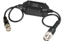
The **VIDGL** Video Ground Loop Isolator is a passive device which reduces ground loop interference within CCTV signals. The **VIDGL** is useful where a video signal is transmitted via cable between points with different ground potentials (typically caused by unbalanced power line loads.)
