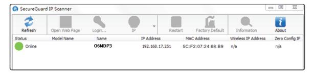
③ In the device list, the IP address, model number, and MAC address of each device will be listed. Select the applicable device and double click to open up the web viewer. You can also manually enter the IP address in the address bar of the web browser.
