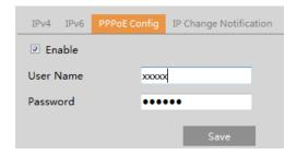
Either method of network connection can be used. If PPPoE is used to connect internet, the camera will get a dynamic WAN IP address. This IP address will change frequently. To be notified, the IP change notification function can be used. Click "IP Change Notification Config" to go to the interface as shown below.
