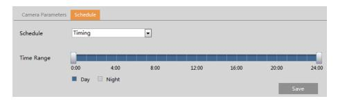
Drag "\bigcapsilon" icons to set the time of day and night. Blue means day time and blank means night time. If the current mode of camera parameters is set to "Timing", the image configuration mode will automatically switch between day and night according to the schedule.
