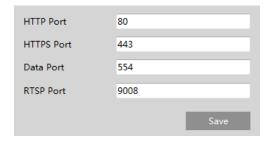
**HTTP Port**: The default HTTP port is 80. It can be changed to any port which is not occupied. **HTTPS Port**: The default HTTPs port is 443. It can be changed to any port which is not occupied.
