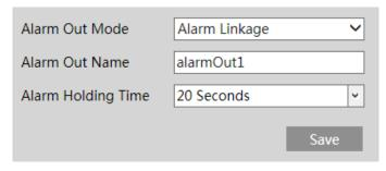
Alarm Out Mode: Alarm linkage, manual operation, day/night switch linkage and schedule are optional.
