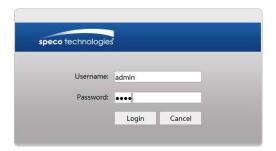
The login interface is shown above. Default user name is admin and password is 1234. After logging in, follow directions to install applicable plug-ins for viewing video.
