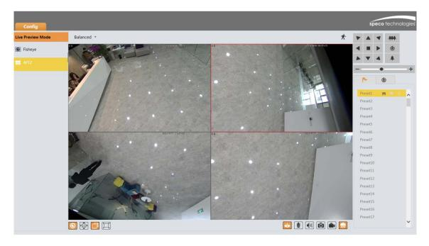
In panoramic + 3PTZ view mode or fisheye + 3PTZ view mode or 4PTZ view mode, select a PTZ window and view the image from every direction by controlling PTZ panel.
