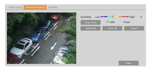
Move the "Sensitivity" scroll bar to set the sensitivity. Higher sensitivity value means that motion will be triggered more easily. Select "Add" and click "Draw". Dragthe mouse to draw the motion detection area; Select "Erase" and dragthe mouse to clear motion detection area.
