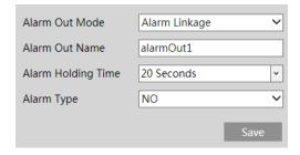
Alarm Out Mode: Alarm linkage, manual operation, day/night switch linkage and timing are optional.
