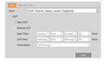
Select the applicable time zone and enable / disable DST as needed. Click the "Date and Time" tab to set the time and date.
