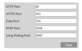
HTTP Port: The default HTTP port is 80. It can be changed to any port which is not occupied.
