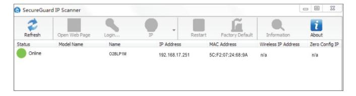
③ In the device list, the IP address, model number, and MAC address of each device will be listed. Select the applicable device and double click to open up the web viewer. You can also manually enter the IP address in the address bar of the web browser.
