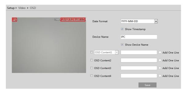
Set time stamp, device name, OSD content and picture overlap here. After enabling the corresponding display and entering the content, drag them to change their position. Then click the "Save" button to save the settings.
