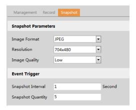
Set the format, resolution and quality of the image saved on the SD card and the snapshot interval and quantity and the timing snapshot here.
