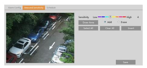
Move the "Sensitivity" scroll bar to set the sensitivity. Higher sensitivity value means that motion will be triggered more easily. Select "Add" and click "Draw". Drag the mouse to draw the motion detection area; Select "Erase" and drag the mouse to clear motion detection area.
