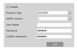
To use this function, the camera shall be connected to a switch supporting 802.1x protocol. The switch can be reckoned as an authentication system to identify the device in a local network. If the camera connected to the network interface of the switch has passed the authentication of the switch, it can be accessed via the local network.
