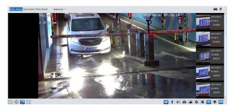
When the captured license plate is matched with the license plate of the comparison list, the list type will be displayed under the license plate number. Click the matched license plate picture, the matched details will pop up as shown below.
