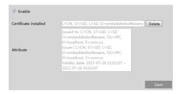
There is a certificate installed by default as shown above. Enable this function and save it. Then the camera can be accessed by entering https://IP: https://IP:
