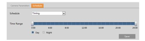
Drag "\bigcolor" icons to set the time of day and night. Blue means day time and blank means night time. If the current mode of camera parameters is set to "Timing", the image configuration mode will automatically switch between day and night according to the schedule.
