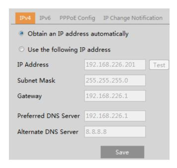
**Use IP address (take IPv4 for example)**-obtain a local IP address automatically through DHCP. A typical router has a DHCP server built in, and therefore is able to assign an IP address to the camera.
