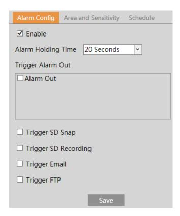
1. Check "Enable" check box to activate motion based alarms. If unchecked, the camera will not send out any signals to trigger motion-based recording to the NVR or CMS, even if there is motion in the video.
