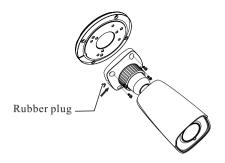
① Connect the cables and then install the camera onto the junction box as shown below.
