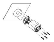
4. Bracket adjustment. Before adjustment, preview the image of the camera on a monitor and then loosen the fixed ring to adjust the view angle of the camera. Tighten the fixed ring after the adjustment.
