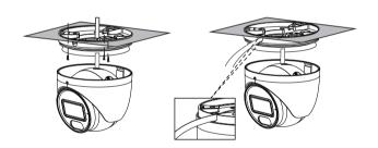
4. Install the dome and enclosure to the mounting base.
