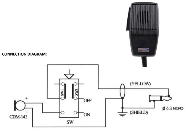
NOTE ON SWITCH TIMING: When Push to talk switch is pressed, SW2 contact closes before SW1 contact closes.
