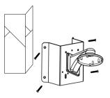
4. Srew the mounting base of the dome camera to the wall mount with screws.
