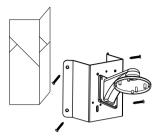
4. Srew the mounting base of the dome camera to the wall mount with screws.
