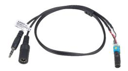
Thank you for your purchase of the **CAMMICV** mini microphone with volume. This microphone is line level and ideal for use with surveillance cameras or recorders. The volume adjustment is perfect for installations where feedback is a risk, or if there is a lot of background noise and you want the pickup to be closer to the microphone.
