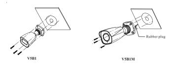
4. Bracket adjustment. Before adjustment, preview the image of the camera on a monitor and then loosen the fixed ring to adjust the view angle of the camera. Tighten the fixed ring after the adjustment.
