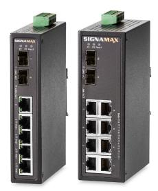
Their extended temperature ranges from -40°F to 167°F (-40°C to 75°C). Both switches are offered in a compact, all-metal IP30 case with built-in DIN-rail mounting. The advantage of PoE+ support allows these switches to handle Pan/Tilt/Zoom for IP security camera requirements.
