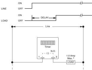
For higher current applications connect a switching relay in series with timer in place of load. Binary Switch, Programmable, AC, Delay on Operate, Solid State, Universal Cube Timer.
