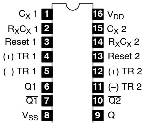
**Note:** Pin1, Pin8, and Pin15 are electrically connected internally
