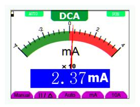
Figure 8: 400mA DC Current Measurement
