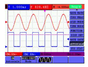
Fig 32: Autoscale Horizontal - Vertical multi-period waveforms
