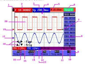
Figure 4: Oscilloscope Display Screen
