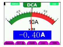
Figure 9: 10A DC Current Measurement
