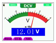
Figure 13: Automatic/Manual Range Adjustment
