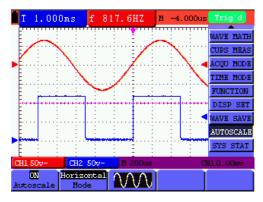
Fig 35: Horizontal mode multi-period waveform
