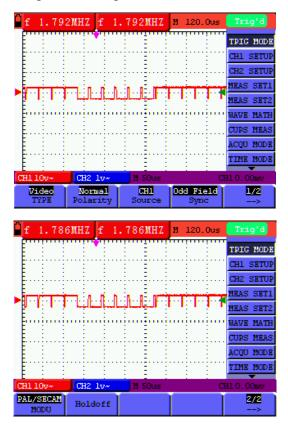
Figure 24a (screen 1) and 24b (screen 2): Odd Field Video Trigger
