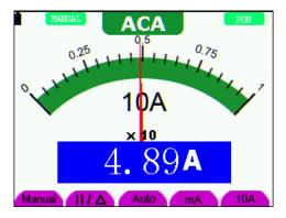
Figure 11: AC Current Measurement for 10A
