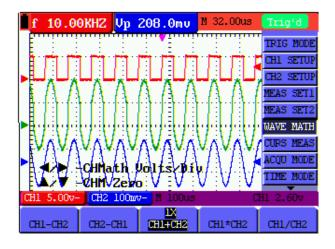
Figure 18: Waveform Mathematical Calculations
