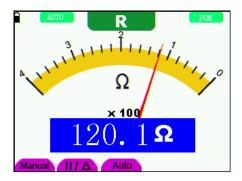
Figure 2: Resistance Measurement
