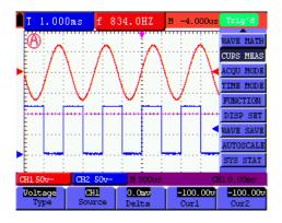
Figure 36-a: Use the Cursor for a Voltage Measurement
