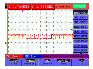
Fig. 25: Video Line trigger (screen 1)
