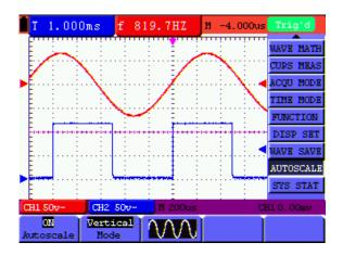
Fig 34: Vertical mode multi-period waveform
