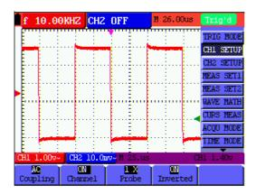
Figure 17: Inverted Waveform
