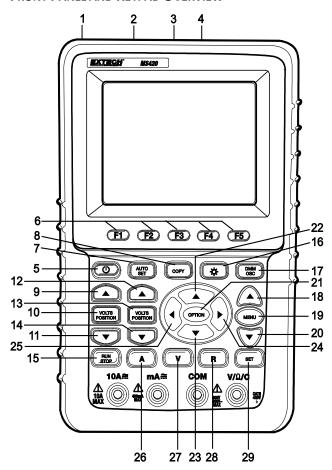
Description of Meter Front Panel and Keypad (Figure 3)
