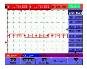
Fig. 26: Video Line Trigger (screen 2)
