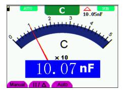
Figure 5: Capacitance Measurement
