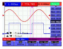
Figure 37-a: Time Measurement using cursor
