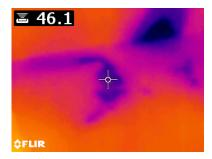
Fig. 5-9(b) Saved image with Target area and Moisture reading
