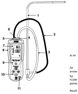
SETUP T: Momentary key presses turn the backlight on and off. Press and hold this button for 3 seconds to enter or exit the Setup mode (discussed later in this guide)
