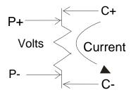
Rx = Vx / Is Where: Vx is the voltage drop across the device under test; Is is the test current; Rx is the resistance of the device under test.
